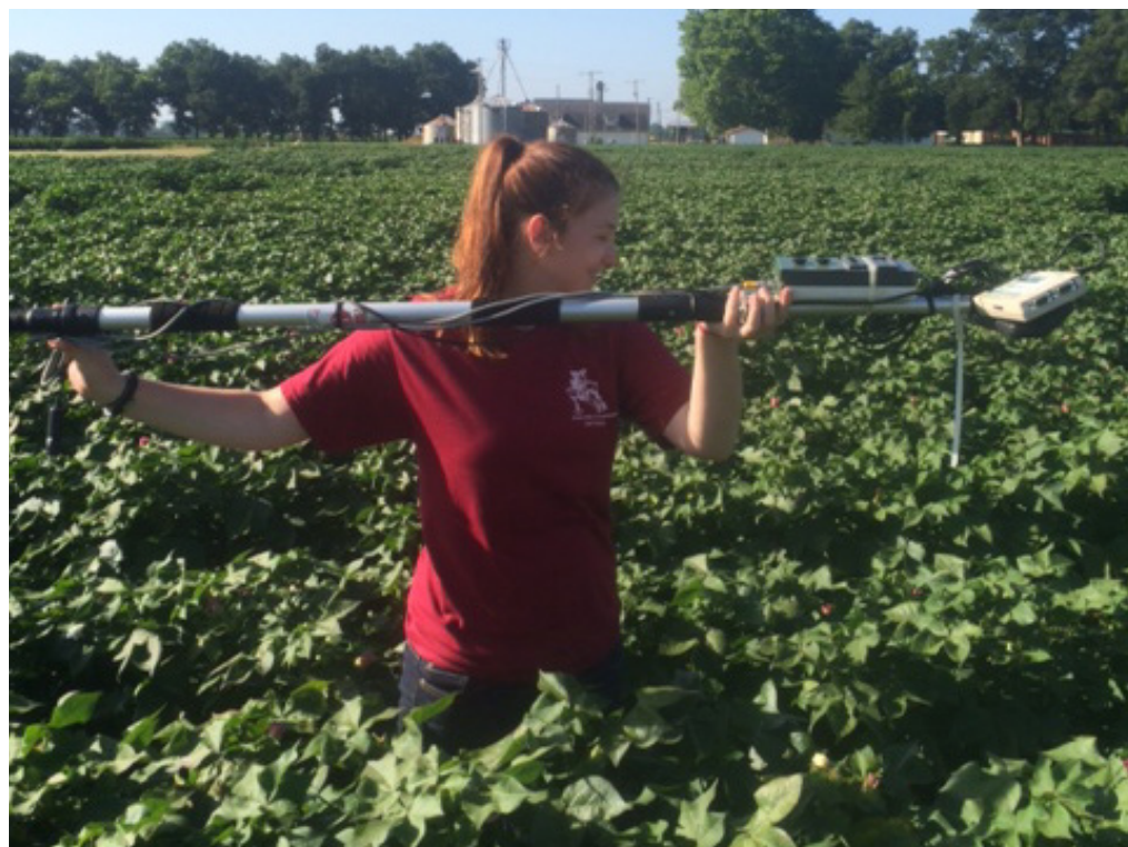
Figure 2. Collecting sensor reflectance data in the cotton field.
