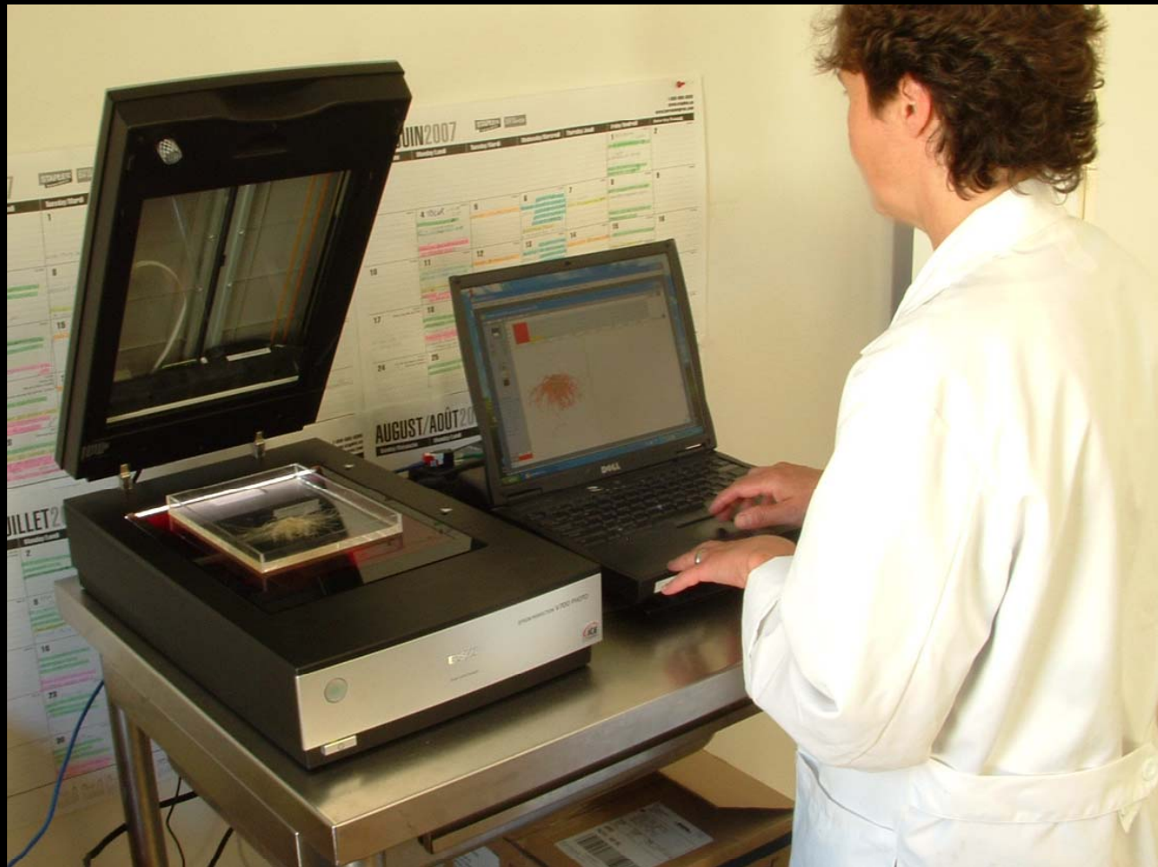
Figure 1. WinRhizo root scanner and associated computer software analyze plant roots for important characteristics of root physiology such as root surface area, root diameter, root volume, and the number of root tips. .
