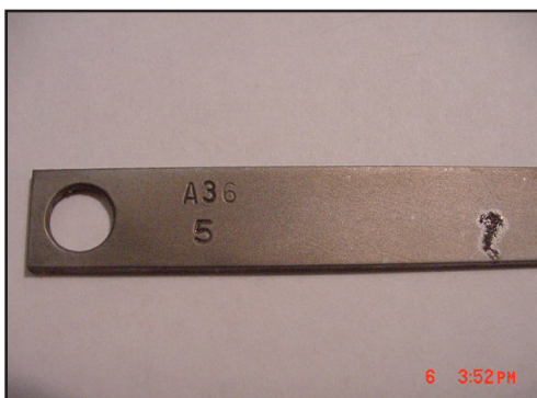
Figure 5. Surface corrosion initially results in minimal damage.
