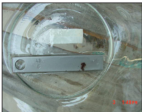
Figure 3. Sealed jar left in sun for 7 days.
