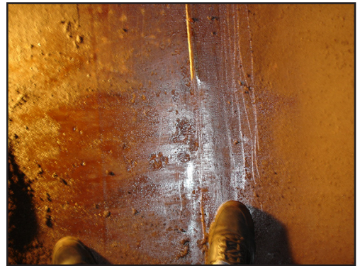
Figure 9. Pitting under UAN rail car sludge.
