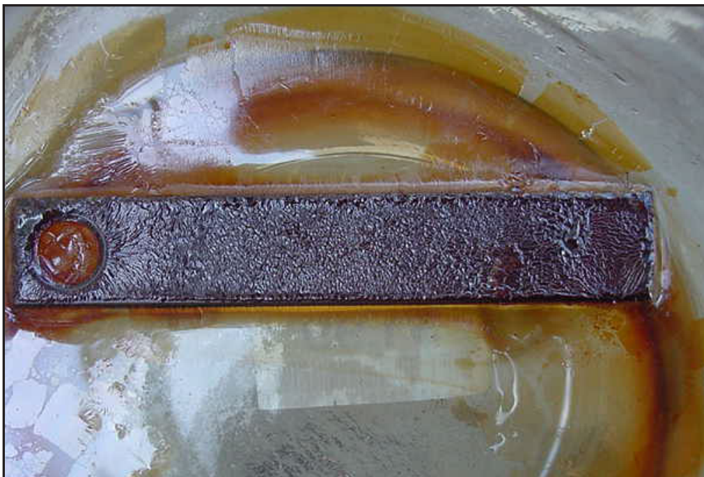
Figure 4. Severe corrosion developed on coupon after loss of ammonia.
