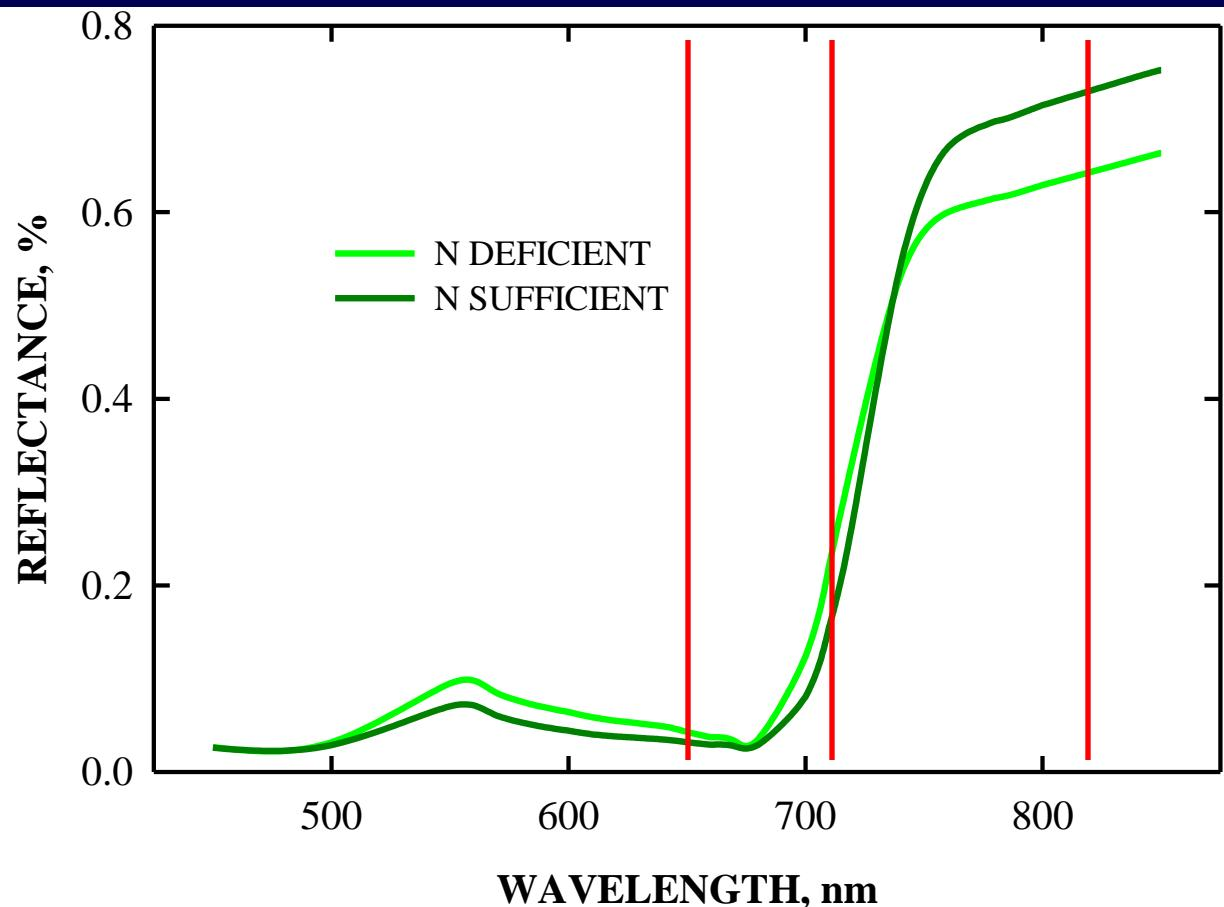
$$NDVI = \frac{R_{NIR} - R_{RED}}{R_{NIR} + R_{RED}}$$
