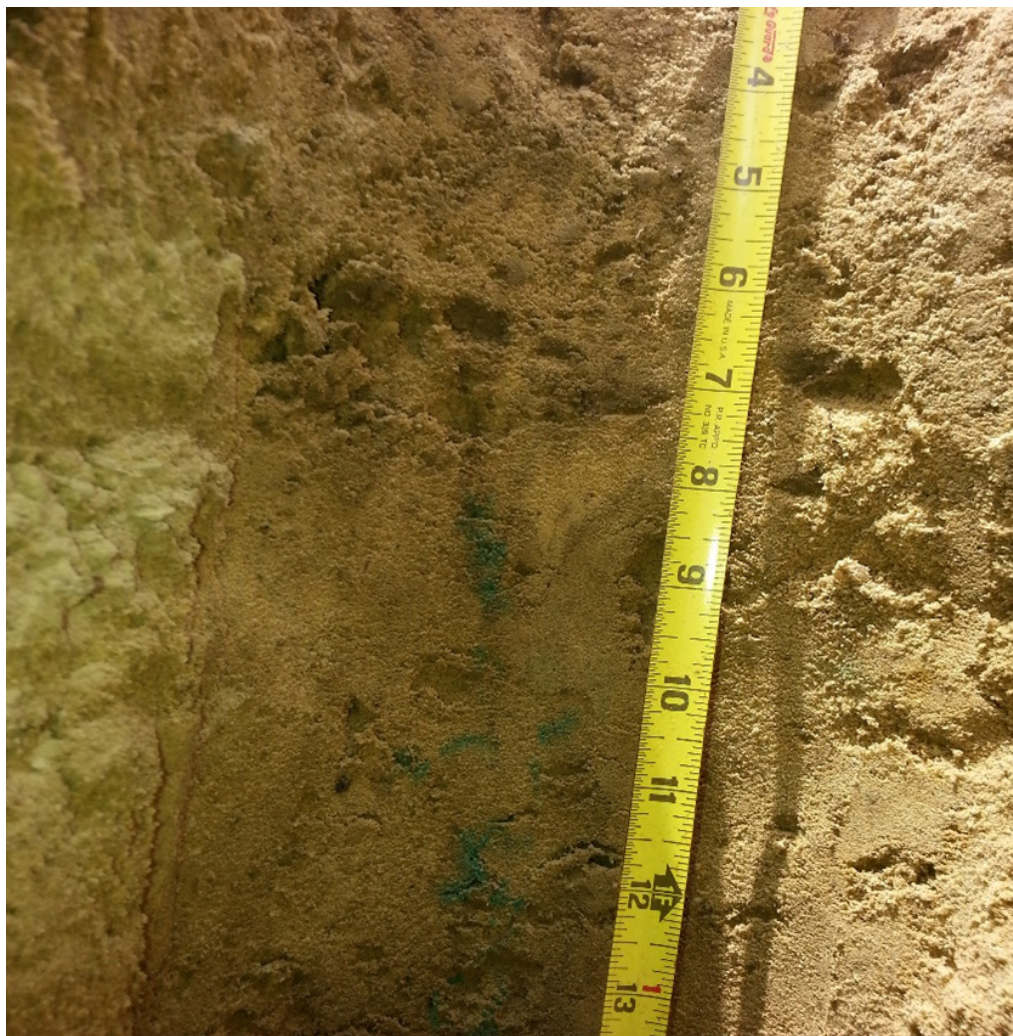
Fig. 2: Demonstration of fertilizer placement with two row strip-tillage implement showing the accuracy of fertilizer (blue dye) placement with the developed applicator.
