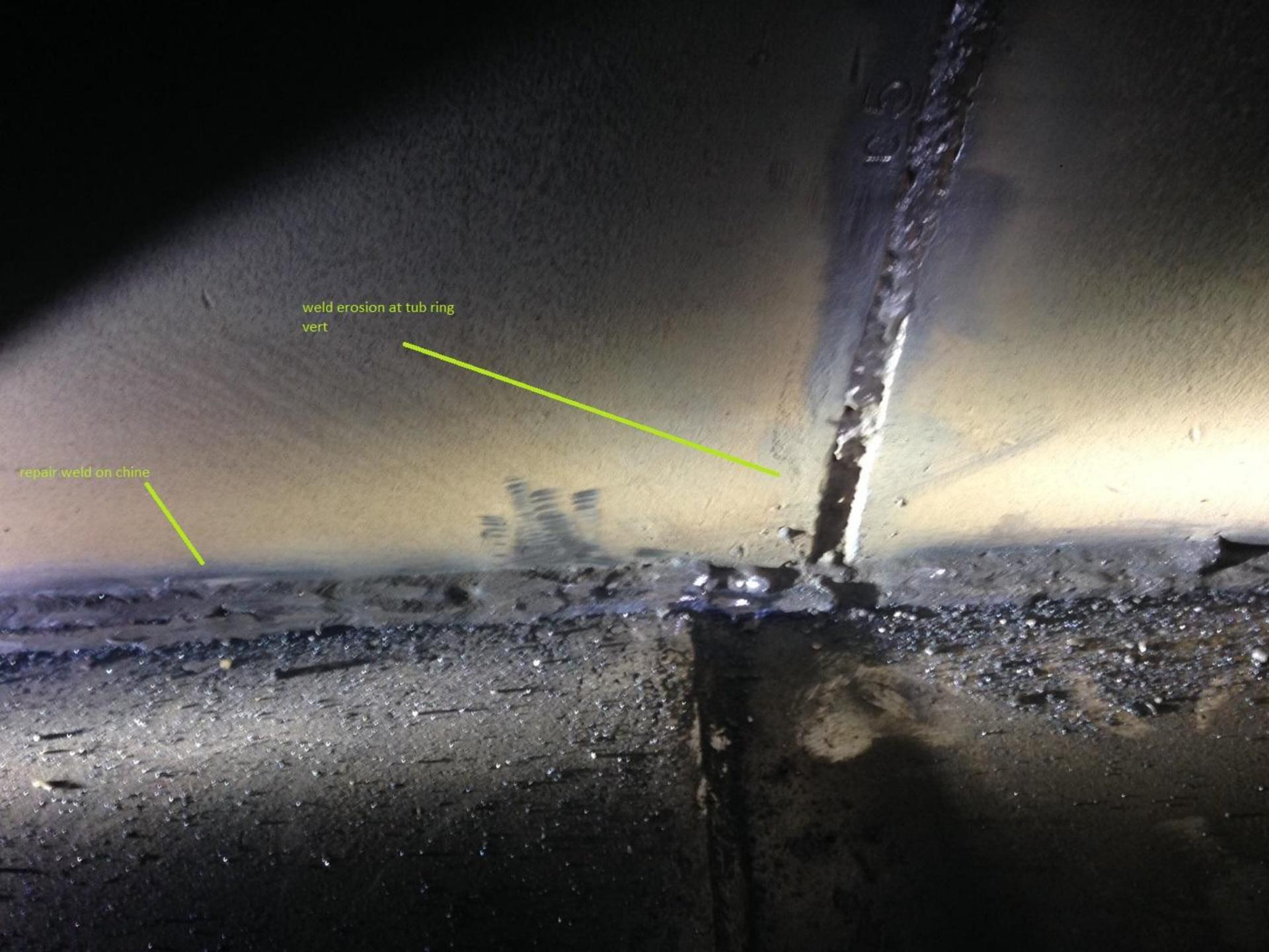
weld erosion at tub ring
