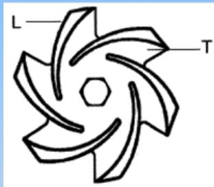
The fluid enters the eye of the impeller where the turning vanes add energy to the fluid and direct it to the discharge nozzle. A close clearance between the vanes and the pump volute, or back plate in a few designs, prevents most of the fluid from recirculating back to the eye of the impeller.
