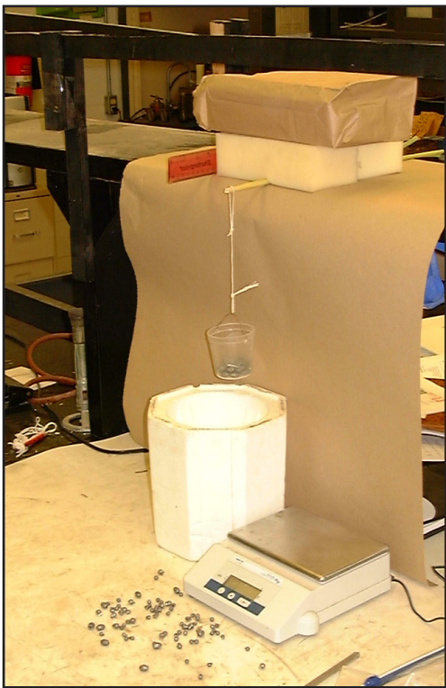
Figure 1. Apparatus used to measure rice stalk breaking strength.
