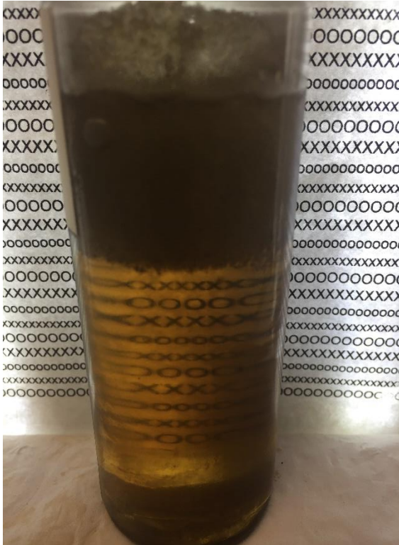
6-24-6 80% Ortho Phosphate In freezer 4 °F for 2 weeks. Note the ice on top and MAP & DAP crystals on the bottom.
